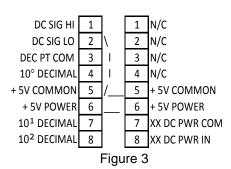
**Decimal Point:** Jumper between terminal 3 and terminal 4, 7 or 8 on the lower terminal block, depending upon which decimal point is to be displayed.
